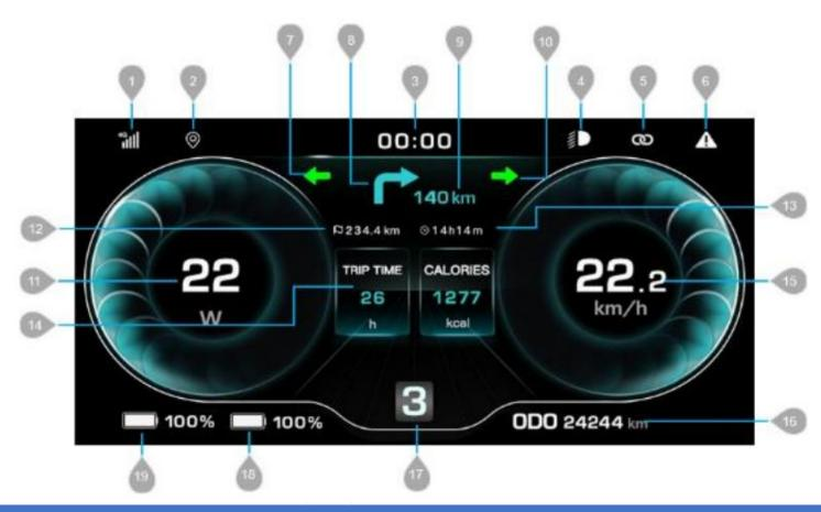
(1) 4G signal GPS sign Time Headlight status (6) Abnormal warn Bluetooth connection sign (7) Turn left 8 Navigation Mileage remaining from current route (1) Turn right (1) Real-time motor power Mileage remaining from destination Time remaining from destination (17) Assist level (14) Riding data (15) Real-time speed (16) ODO (18) Main battery (19) Secondary battery
